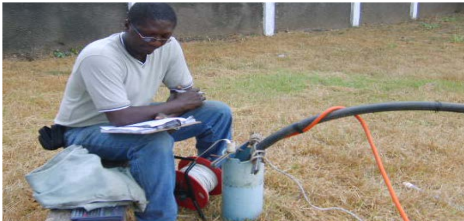
Figure 16: Conducting Pumping test
